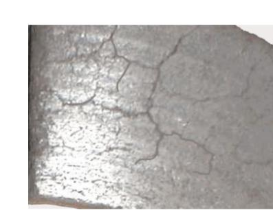
Pad with surface cracks.
