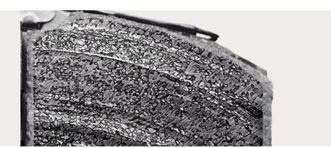
Contaminated pad friction material
