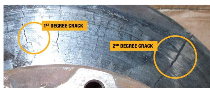
Disc surface features 1st and 2nd degree crack.
