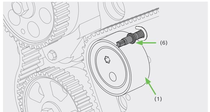
Install the tensioner pulley (1) using the M10 x 45 bolt (5) onto the engine housing:
