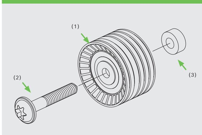
The new idler pulley can differ from the unmounted one. It is installed using the M10 x 66 bolt (2) and the bushing (3) included in the kit.
