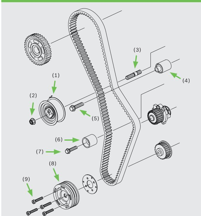
The tensioner pulley (1) is installed onto the stud (3) by means of the M 8 x 1.25 nut (2). The idler pulley (4) is installed using the M 8 x 1.25 x 45 bolt (5), the idler pulley (6) using the M 10 x 1.25 x 26 bolt (7).
