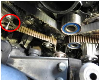
1. Turn the camshaft in the normal direction of rotation
