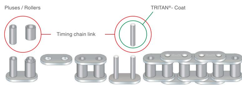
Timing chains, designed as bush chains or roller chains, consist of an arrangement of inner and outer chain links. In this case, pins and bushes form the joint surfaces.
