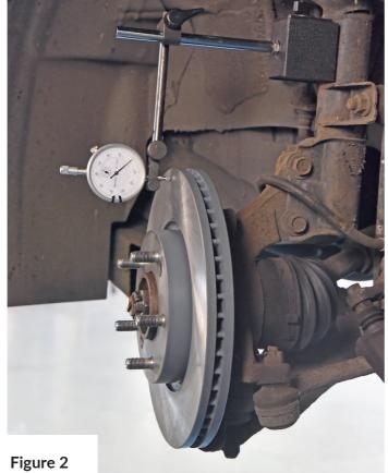
Brake disc 'run-out' must be checked with a dial gauge (Fig 2) with the brake disc secured to the hub, taking note of the point of maximum variation. The utmost recommended 'run-out' is 0.10mm - however, this number may be lower subject to the vehicle manufacturer's specification.
