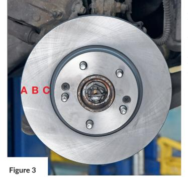
D.T.V. of the brake disc can also be measured separately using a micrometer; the measurements should be taken at points A, B, and C
