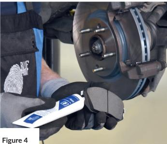
Avoid excessive or high-speed braking until the brake pads and disc are bedded in – a mileage of 150-200 miles (250-300 km) is recommended. Excessive harsh braking during this period can cause heat spots with a consequent reduction in braking efficiency. Remember that brake discs and pads are safety critical components and regular inspection is essential for the safety of the vehicle owner and other road users.
